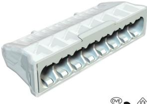
Screwless terminal to connect single-strand cables. Nominal cross-section 2.5  $\div$  mm<sup>2</sup> Rated voltage450 V Rated current24 A 8 x 0.5 mm<sup>2</sup> to 2.5 mm<sup>2</sup> single-wire cables
