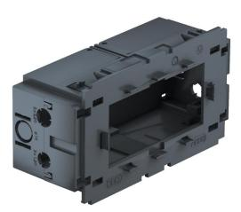
Front locking double accessory mounting box for Modul 45® system, with folding, and also removable, base for time-saving cable connection, with feed openings for cable diameters of up to 14 mm.
