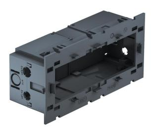
Front locking triple accessory mounting box for Modul 45® system, with folding, and also removable, base for time-saving cable connection, with feed openings for cable diameters of up to 14 mm.
