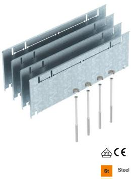
Height compensation set for underfloor boxes UZD350-3 with a construction height of 115 to 170 mm, consisting of four fall plates, four height adjustment screws and four rotary locks.
