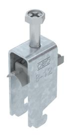
Clamp clip with N-foot, plastic pressure sleeve made of polypropylene. For vertical and horizontal mounting of 2 single cables on a C-profile rail. For slot width 11–12 mm With 1-start screw thread on pressure sleeve, universal hexagonal screw head WAF10, with slot and cross recess. Suitable for assembly indoors and outdoors. Multiple cables should be separated by double sleeves. We recommend the use of a counter-sleeve.
