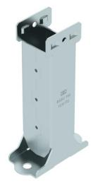
Base of the symmetrical floor support for the BKRS system, suitable for crossbeam type BSST 100. Can be used for walkable cable trays of width 100 mm. With threaded unions for mounting connection components, e.g. pipe clamps, as well as slots for floor mounting up to M10. Fastening material must be ordered separately.
