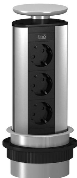
Lowerable Deskbox with connection cable for fixed installation on a tabletop, plastic fastening sleeve, painted accordingly in cover shade. It is mounted using a drill hole (Ø102 mm) in the tabletop.
