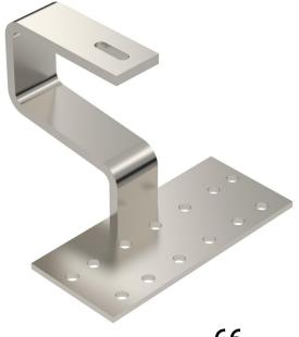
Heavy roof hook to mount photovoltaic modules on pitched roofs in combination with the TP 45 support profile. Suitable for tiled roofs. Fastening on support profile through bolt with hammer nut, type SKSHM A2. Mounting on rafters with TKS wafer-head screws.
