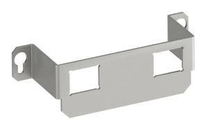
Mounting support to accept two data connection modules of the following types: Brand-Rex: shielded; EKU: E-Stone; Dätwyler: KS-T, MS-K and KU-T module; R&M: Snap-In and Keystone; Rutenbeck: UM and UMflex; SETEC: MKJ, UKJ and XKJ; Siemon TERA; Telegärtner: AMJ and UMJ.
