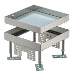
"Blank" height-adjustable cassette for the creation of an inspection opening of nominal size 4. Installation of devices in duct systems, raised and cavity floors in interior dry or wet-care floors. Only suitable for smooth floor coverings. Protection class: IP X5.
