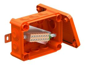
Connection box for data technology with soft plug-in seals. Pairs of high-temperature-resistant ceramic terminals, suitable for data cables. Green-yellow labelled protective conductor/shield terminal. Fastening on easily accessible external flaps. Approved for cable systems that maintain the electrical function according to DIN 4102 Part 12 with the classes E30, E60 and E90. Ceramic clamps have been tested according to DIN EN 60998-2-1:2004.
