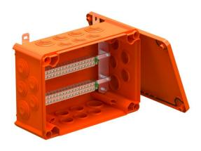
Connection box for data technology with soft plug-in seals. Pairs of high-temperature-resistant ceramic terminals, suitable for data cables. Green-yellow labelled protective conductor/shield terminal. Fastening on easily accessible external flaps. Approved for cable systems that maintain the electrical function according to DIN 4102 Part 12 with the classes E30, E60 and E90. Ceramic clamps have been tested according to DIN EN 60998-2-1:2004.
